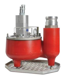
This submersible centrifugal design requires no priming and can run dry all day without damage. Direct drive requires no maintenance as all moving parts are self lubricated with passing hydraulic fluid. A urethane bowl and impeller are very durable and capable of moving liquids containing up to 30% solids. If you are pumping oily sludge, septic systems, muddy trenches or even clean water this a pump for you.
