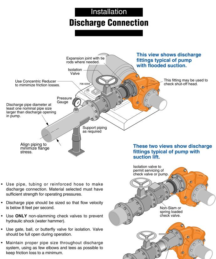
Install pressure gauge after reducer as shown to • check operating pressure or shut-off head.
