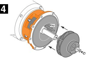
impeller on to shaft as far as possible.
