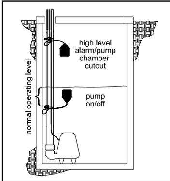
**FIGURE 6 - Sand filter redundant off system**
