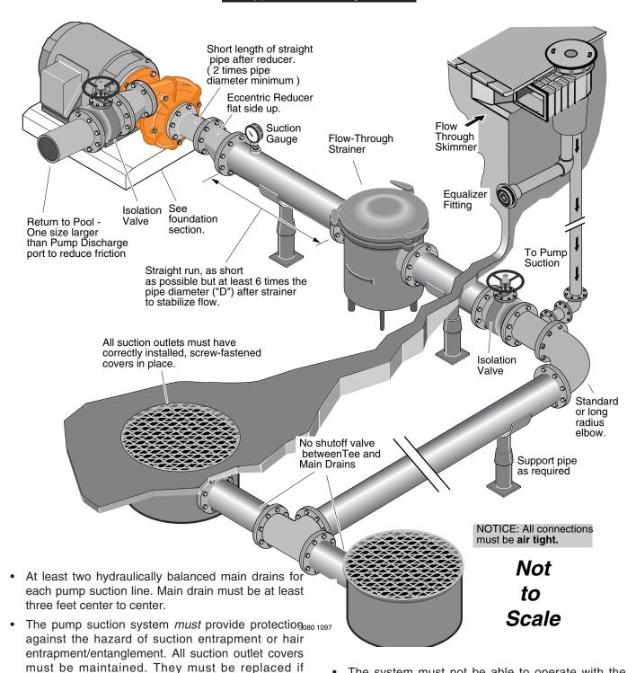
The system must not be able to operate with the pump drawing water from only *one* main drain (that is, there must be at least two main drains connected to the pump suction hydraulic system must be six feet per second or less even if one main drain (suction fitting) is completely blocked.
