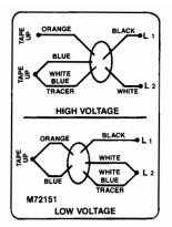
NOTE: Single phase motors are protected with inherent overheating devices and do not require external overload protection.
