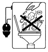
objects like fruit pits, rags, wet strength kitchen towels, tampons or sanitary napkins. The holding tank and pump should be flushed with several gallons of water after each pumpout. Make sure the battery is fully charged. The dc motor is suitable only for intermittent duty and should not be run for more than 15 minutes continuously. At maximum flow of 12 GPM (45 LPM) the macerator can empty a 180 gallon (680 liter) holding tank in a single operation.
