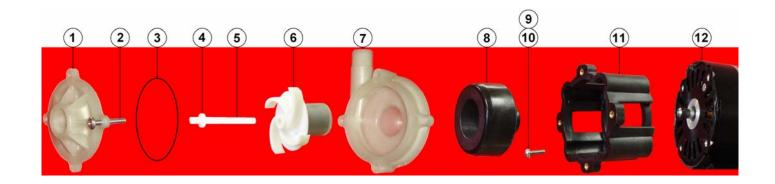
**NOTE:** WHEN ATTACHING DRIVE MAGNET (ITEM 8) TO THE MOTOR SHAFT. POSITION THE FACE OF THE DRIVE MAGNET 3/32 INCH BELOW THE FACE OF THE MOTOR BRACKET (ITEM 11).
