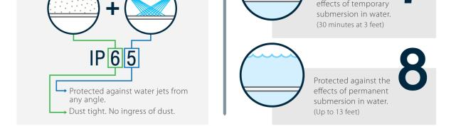
Example: With an IP65 rating, the LEDs can be used in an outside setting and are water-resistant but they are not waterproof and are not suitable to be submerged. An IP68 can be submerged in water.
