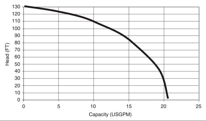
EBG-31 EBG-33 (3HP) Synchronous Speed: 3450 RPM 21/2 / 3 inch Discharge
