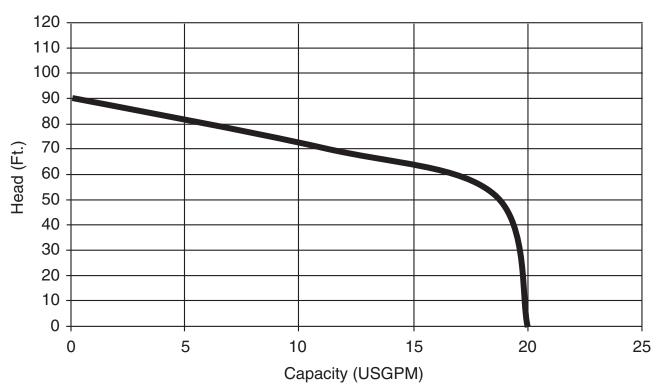
EBG2-212C (2HP) Synchronous Speed: 3450 RPM 11/4 inch Discharge
