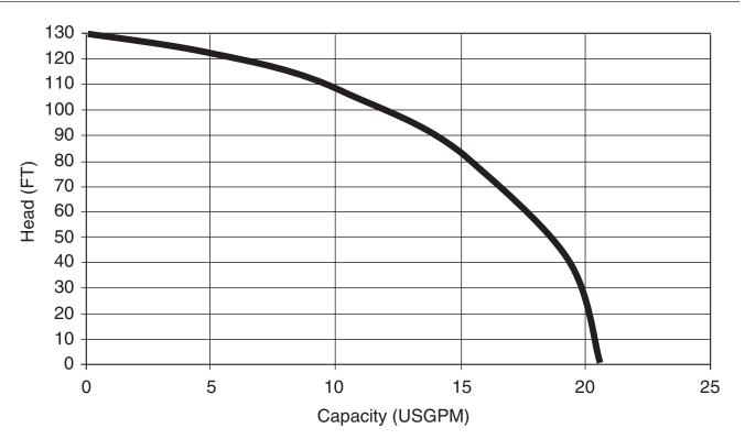
EBG2-21 EBG2-23 (2HP) Synchronous Speed: 3450 RPM 11/4 inch Discharge
