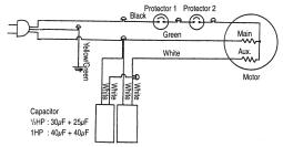
Output ½ to 1 HP (0.4kw to 0.75kw) 230V
